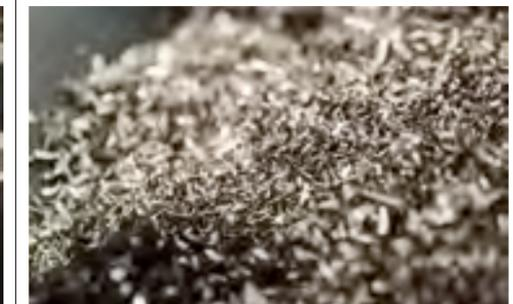
100% of the company's brass waste material, resulting during the machining and grinding process, gets re-melted into brass ingots and recycled to produce new products.
